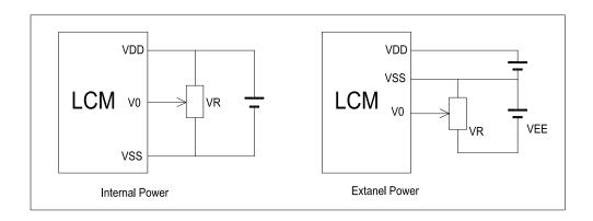
V<sub>DD~</sub>V<sub>0</sub>: LCD Driving voltage
