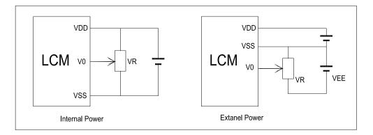
V<sub>DD-</sub>V<sub>0</sub>: LCD Driving voltage VR: 10k~20k
