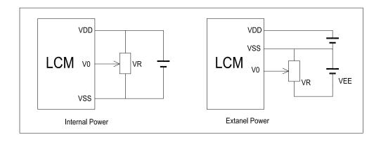
V<sub>DD~</sub>V<sub>0</sub>: LCD Driving voltage VR: 10k~20k
