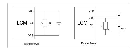
$V_{\text{DD}\text{-}}V_0\text{: LCD}$  Driving voltage
