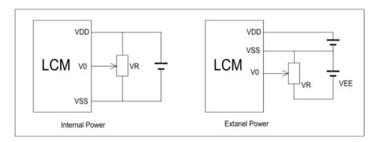
VDD-V0: LCD Driving Voltage VR: 10k-20k
