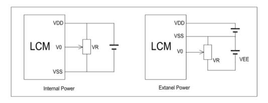
VDD-V0: LCD Driving Voltage
