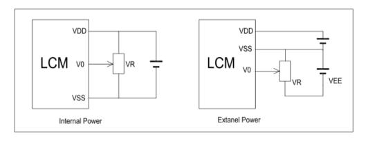
VDD-V0: LCD Driving Voltage
