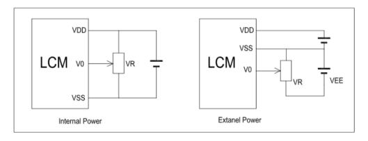
VDD-V0: LCD Driving Voltage
