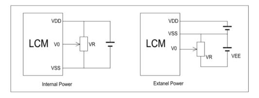
VDD-V0: LCD Driving Voltage
