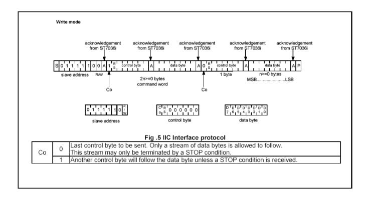
During write operation, two 8-bit registers are used. One is data register (DR), the other is instruction register(IR).
