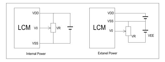
V<sub>DD-</sub>V<sub>0</sub>: LCD Driving voltage VR: 10k~20k
