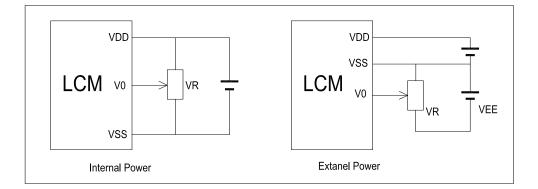
$V_{DD-}V_0$ : LCD Driving voltage VR: 10k~20k
