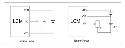
VDD-V0: LCD Driving Voltage
