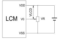
$V_{DD-}V_0$ : LCD Driving voltage VR: 10k~20k
