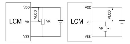
$V_{DD-V_0}$ : LCD Driving voltage VR: 10k~20k
