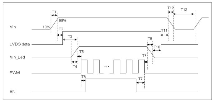
Figure 6.4: Power On/OFF Sequence Timing Diagram
