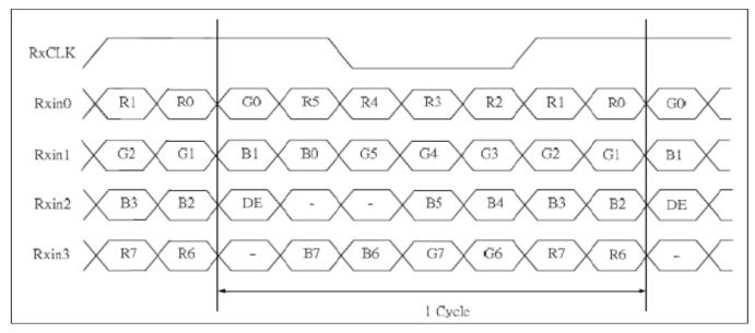
Figure 6.2: RGB Input Data Mapping Timing Diagram
