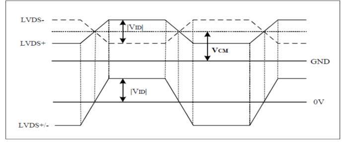
Figure 6.1: LVDS Receiver Differential Input Timing Diagram
