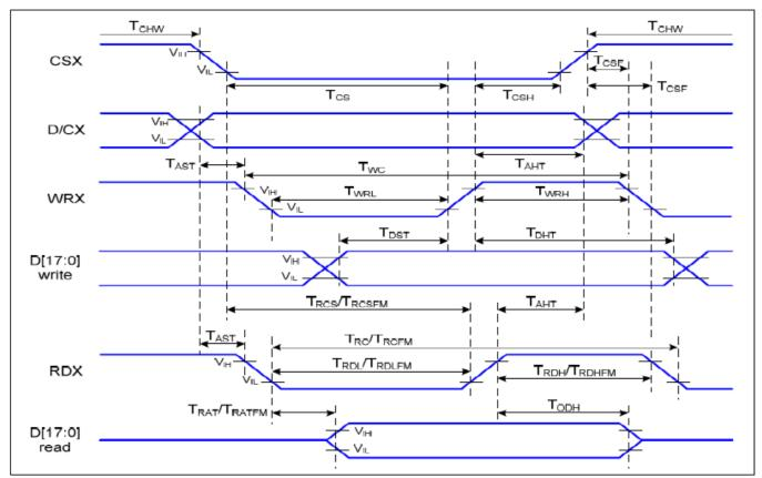
Figure 6.1: 8080 Series MCU Parallel Interface Timing Diagram
