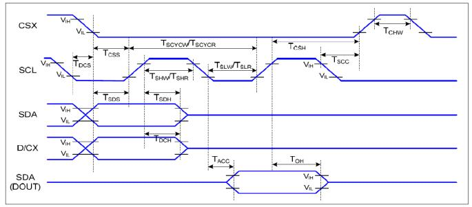
Figure 6.3: 4-line Serial Interface Timing Diagram
