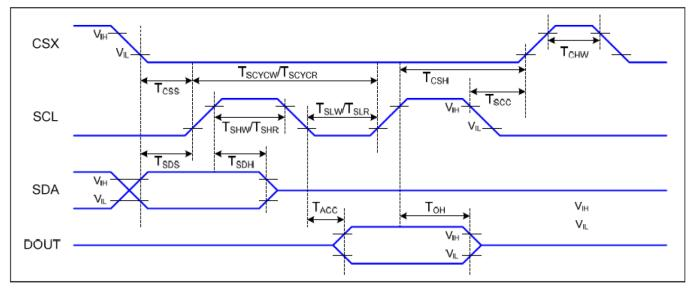
Figure 6.2: 3-line Serial Interface Timing Diagram
