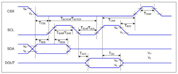
Figure 6.3: Serial Interface 3-SPI Timing Diagram
