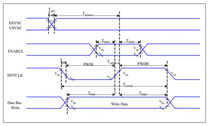
Figure 6.1: RGB Interface Timing Characteristics
