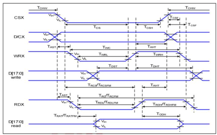
Figure 6.2: Parallel Interface Timing Characteristics (8080-Series MCU Interface)
