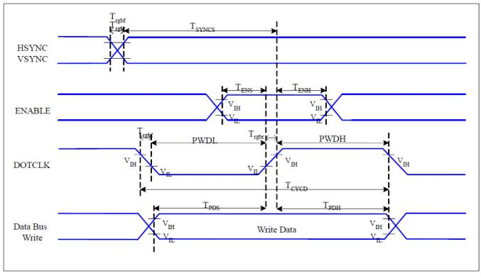
Figure 6.1: RGB Interface Timing Characteristics
