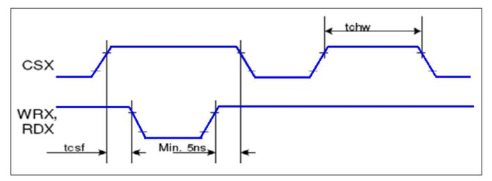
Note: Logic high and low levels are specified as 30% and 70% of IOVCC for input signals.
