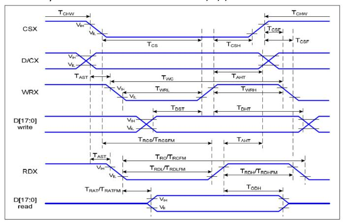
Figure 7.2: Parallel Interface Timing Diagram
