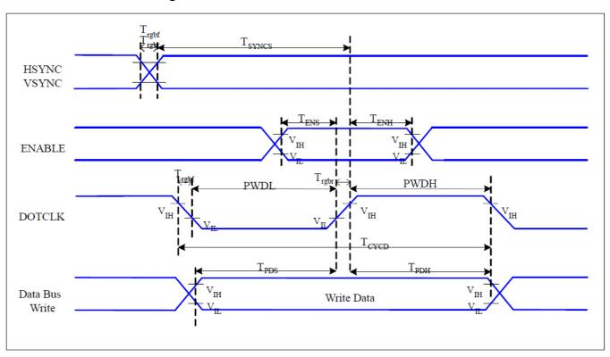
Figure 7.1: RGB Interface Timing Diagram
