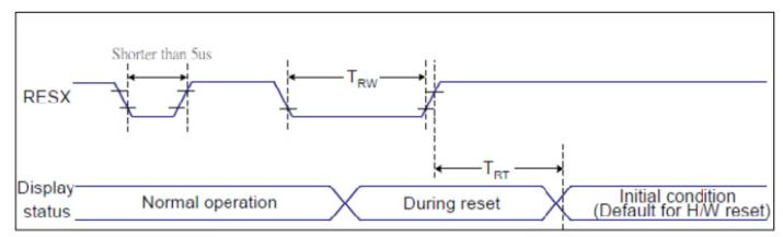
Figure 6.5: Reset Timing Diagram
