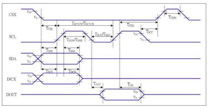
Figure 6.4: 4-Line Serial Interface Timing Diagram
