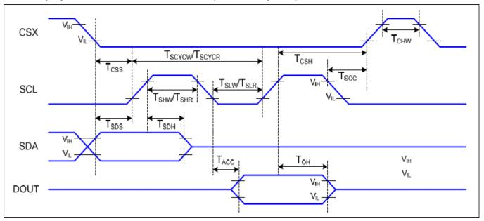
Figure 6.3: 3-Line Serial Interface Timing Diagram
