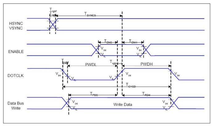
Figure 6.1: Parallel RGB Interface Timing Diagram
