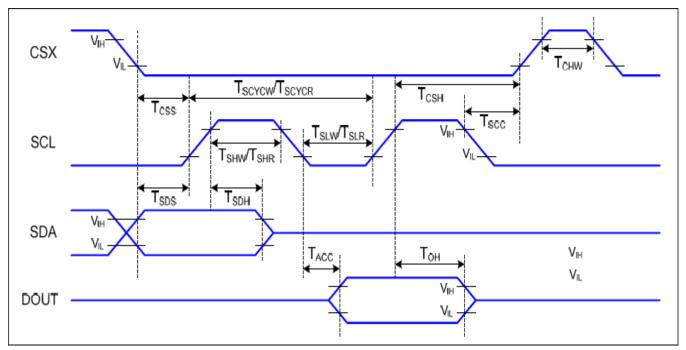
Figure 6.3: Serial Interface 3-SPI Timing Diagram
