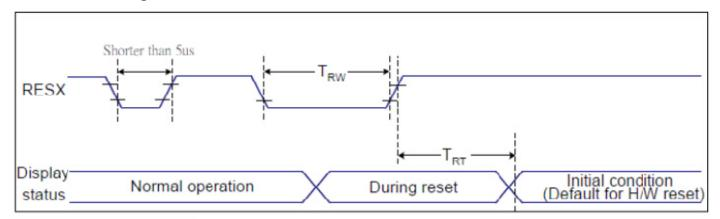
Figure 6.5: Reset Timing Diagram
