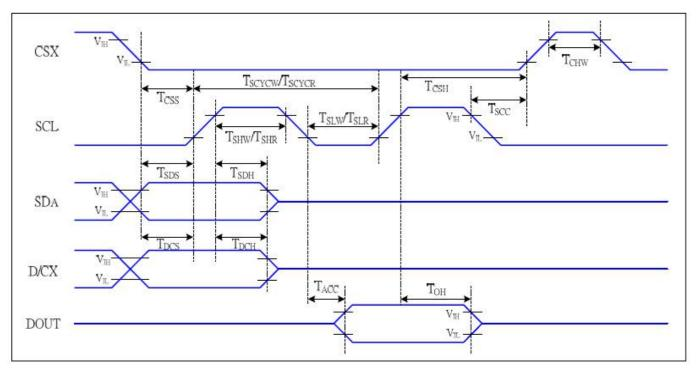
Figure 6.4: Serial Interface 4-SPI Timing Diagram
