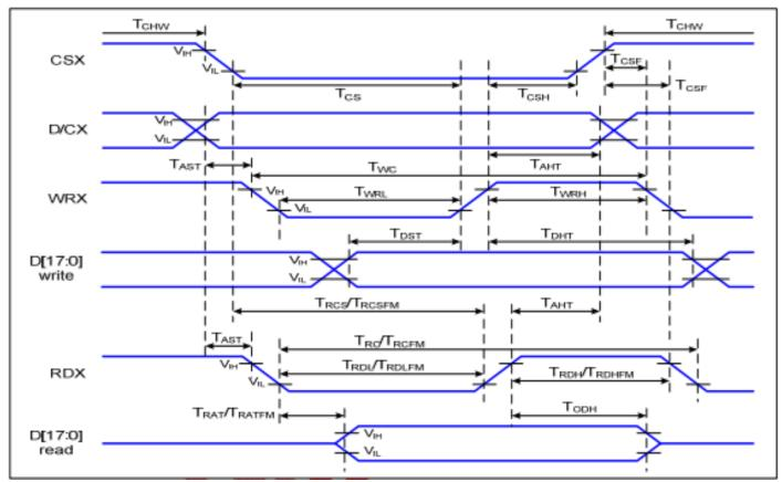
6.5 8080 Series MCU Parallel Interface Characteristics: 18/16/9/8-bit Bus
