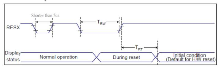
Figure 6.6: Reset Timing Diagram
