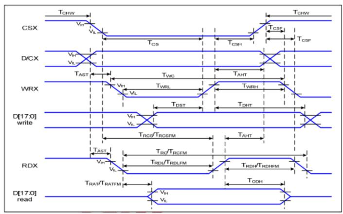
Figure 6.5: Parallel Interface Timing Characteristics (8080-Series MCU Interface)
