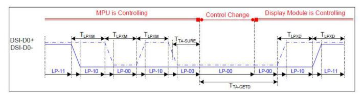
Figure 6.2: Bus Turnaround (BTA) from Display Module to MPU Timing Diagram
