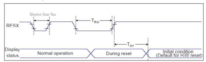
Figure 6.6: Reset Timing Diagram
