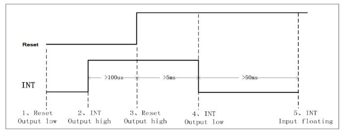
Figure 7.3: Setting Slave Address to 0x28/0x29 Timing
