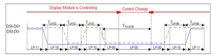
Figure 6.3: Buss Turnaround (BTA) from MPU to Display Module Timing Diagram
