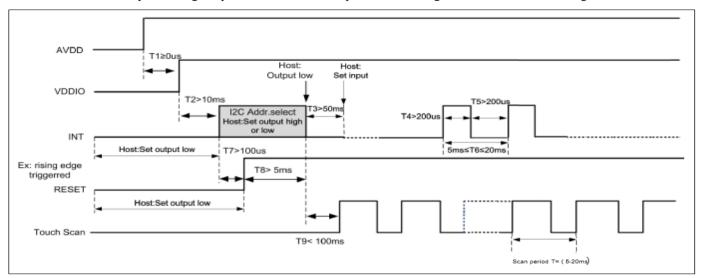
Figure 7.1: I2C Power on Timing
