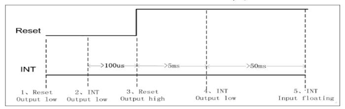
Figure 7.4: Setting Slave Address to 0xBA/0xBB Timing
