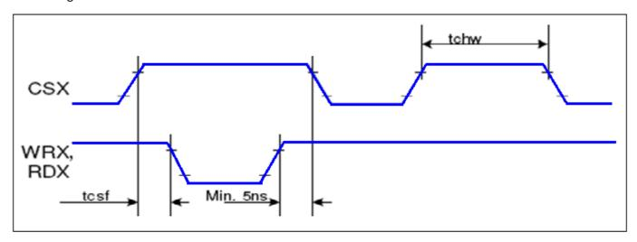
Note: Logic high and low levels are specified as 30% and 70% of IOVCC for input signals.
