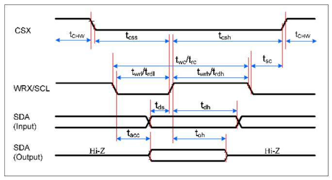
Figure 6.3: 3-line Serial Interface Timing Diagram
