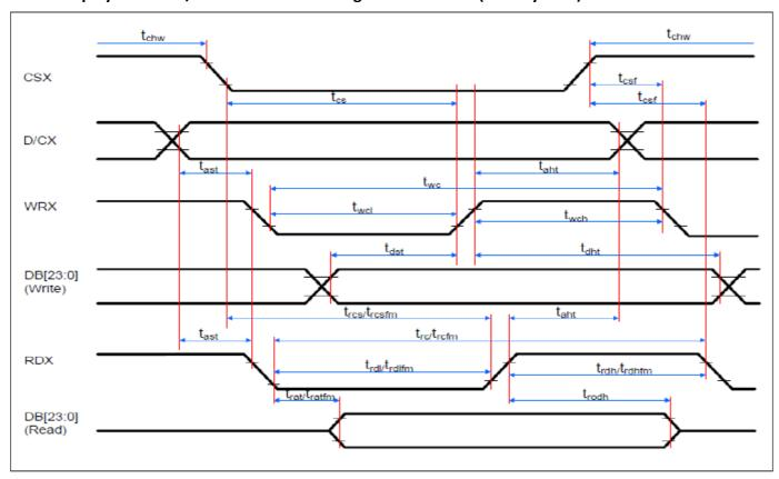
Figure 6.2: 8080 System Parallel Interface Timing Diagram
