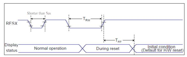
Figure 6.5: Reset Timing Diagram
