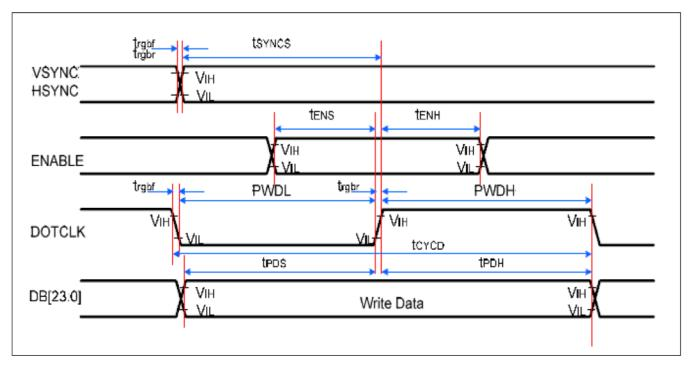
Figure 6.1: Parallel RGB 16/18/24-Bit Timing Diagram
