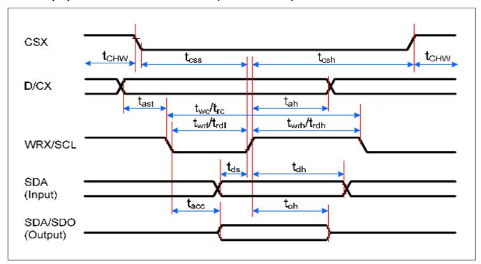
Figure 6.4: 4-line SPI Serial Interface Diagram
