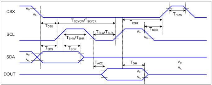
Figure 6.3: 3-line Serial Interface Timing Diagram
