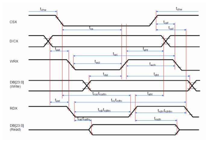
Figure 6.2: Parallel Interface Timing Diagram (8080-Series MCU Interface)
