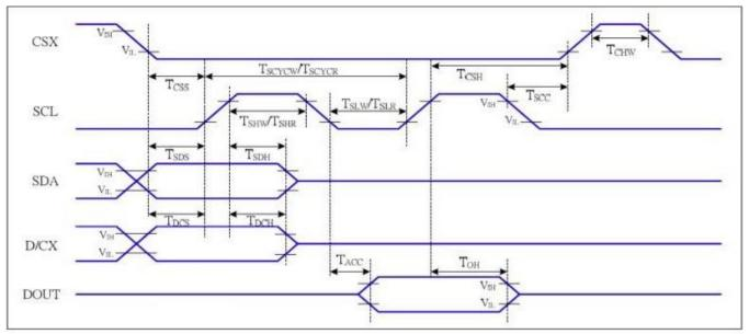
Figure 6.4: 4-line Serial Interface Timing Diagram
