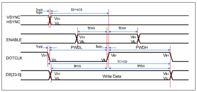
Figure 6.1: Parallel RGB Interface Timing Diagram
