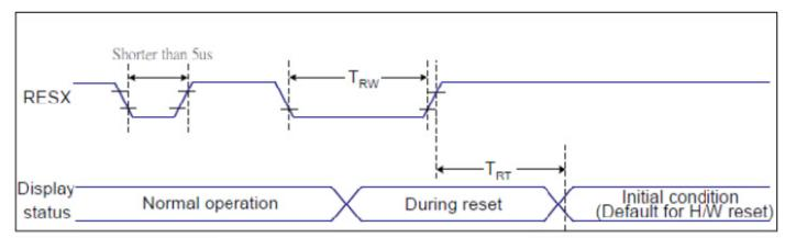
Figure 6.3: Reset Timing Diagram
