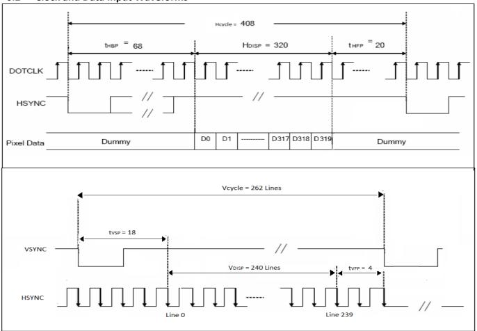
Figure 6.2: Vertical and Horizontal Data Transaction Timing Diagram
