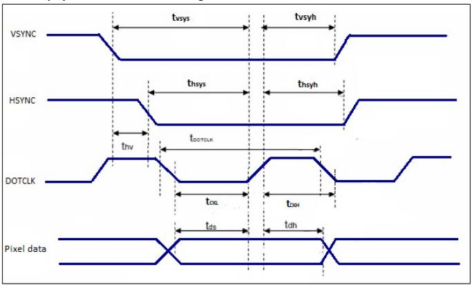
Figure 6.1: Parallel RGB Interface Timing Diagram
