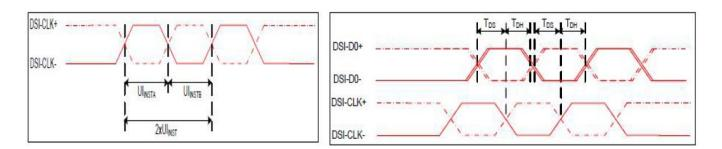
Figure 6.1: DSI Clock Channel Timing Diagram
