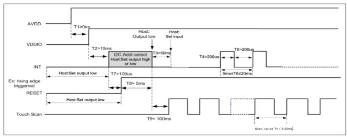
Figure 7.1: I2C Power on Timing
