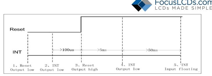
Figure 7.5: Setting Slave Address to 0xBA/0xBB Timing
