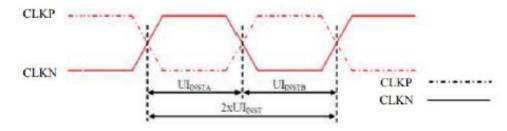
Figure 116: DSI Clock Channel Timing
