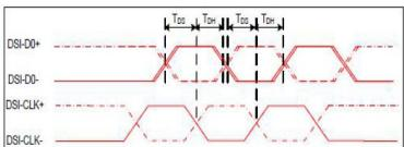
Figure 6.1: DSI Clock Channel Timing Diagram
