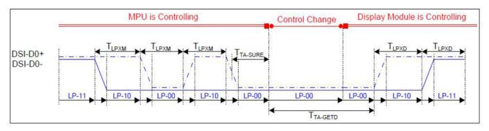
Figure 6.2: Bus Turnaround (BTA) from Display Module to MPU Timing Diagram
