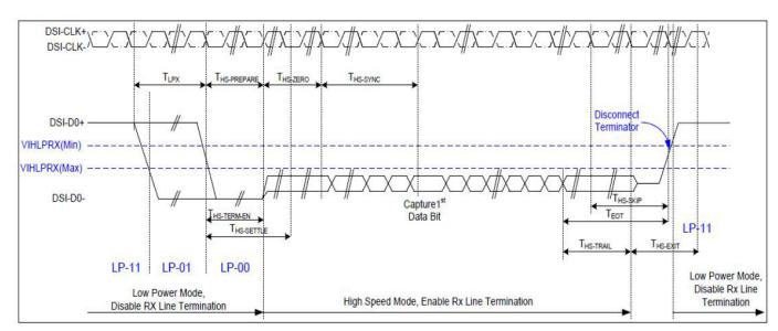
Figure 6.4: Data Lanes Low Power Mode to/from High Speed Mode Timing Diagram
