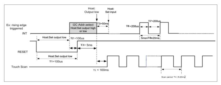
Figure 7.2: I2C Host Resetting Timing
