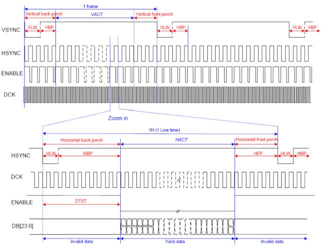
VLW: VSYNC Low pulse Width HLW: HSYNC Low pulse Width DTST: Data Transfer Startup Time Pn: pixel 1, pixel  $2\cdots$ , pixel n.
