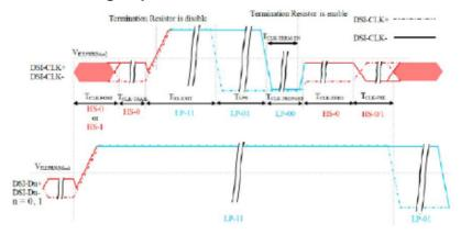
Figure 121 Clock Lanes – High Speed Mode to/from Low Power Mode Timings
