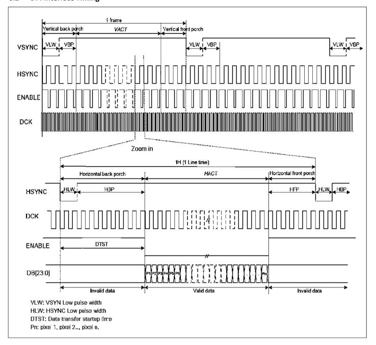
Figure 6.2: Clock and Data Input Timing Characteristics
