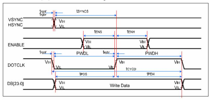
Figure 6.1: 24/18/16 Bits RGB Interface Timing Characteristics
