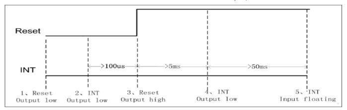
Figure 7.3.4: Setting Slave Address to 0xBA/0xBB Timing
