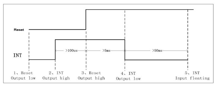
Figure 7.3.3: Setting Slave Address to 0x28/0x29 Timing
