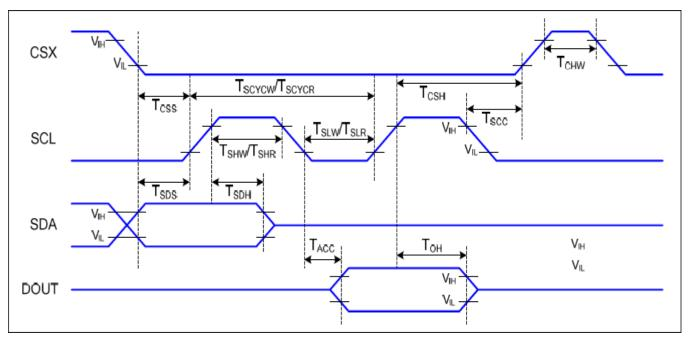
Figure 6.3: 3-line Serial Interface Timing Characteristics
