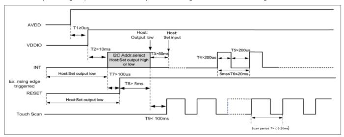
Figure 7..3.1: I2C Power on Timing
