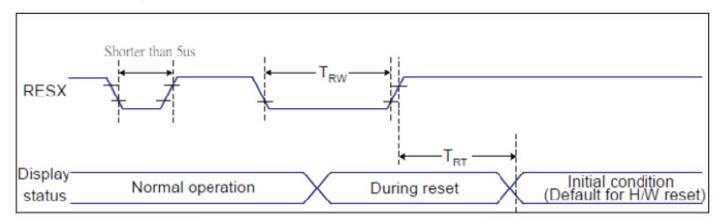
Figure 6.4: Reset Timing Diagram
