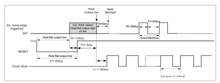
Figure 7.2: I2C Host Resetting Timing
