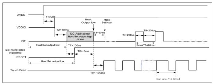
Figure 7.1: I2C Power on Timing
