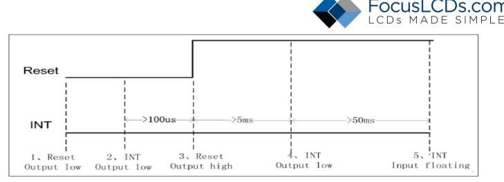
Figure 7.4: Setting Slave Address to 0xBA/0xBB Timing
