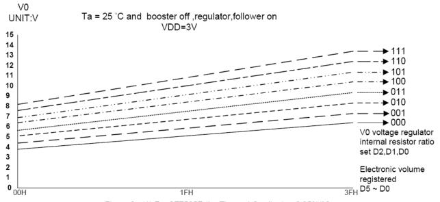
Figure 9 : (1) For ST7565R the Thermal Gradient = -0.05%/ $^{\circ}$ C
