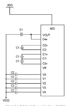
C1: 1uF-4.7uF for Voltage rating from 10-35V C2: 1uF-2.2uF for Voltage rating from 6.3-25V
