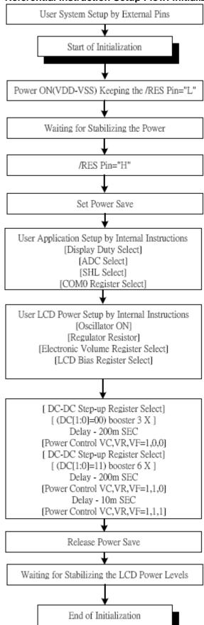
Figure 27 Initializing without Built-in Power Supply Circuits
