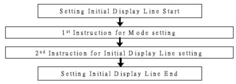
Figure 20 Sequence For Setting Initial Display Line
