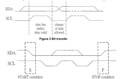
Figure 4 Definition of START and STOP conditions
