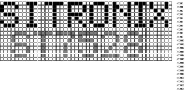
Figure 14 Partial Display (Partial Display ratio=16,initial COM0=0)
