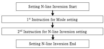
Figure 23 Sequence For N-line Inversion
