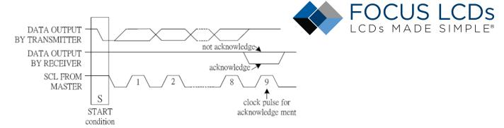
Figure 5 Acknowledgement on the 2-line Interface
